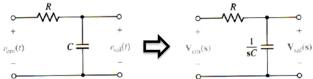
$$V_{sal} = V_{ent} \frac{Z_C}{Z_C + R}$$
