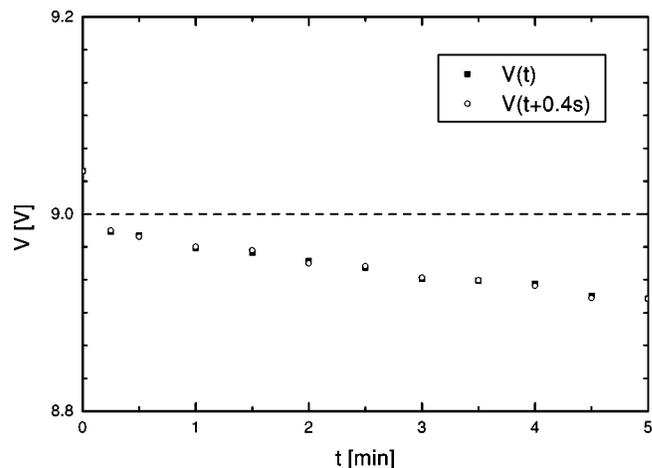
Fig. 4. Measurements of the voltage of the battery over 5 min when a 1 k $\Omega$  load is applied. We take two voltage series,  $V(t)$  and  $V(t+0.4s)$ , to determine if their differences are significant. The dispersion of each point of both data series is 0.002 V and is not plotted in the figure.
