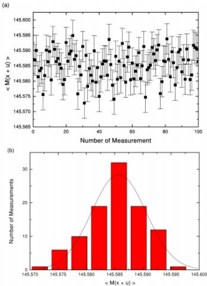
Fig. 1. (a) 100 measurements,  $\langle M(x+u) \rangle$ , obtained by taking the integer part of a real number after adding noise and averaging over 10 000 points, in the order that they were obtained. (In all cases  $S_i \approx 0.5$  and  $S_{N_i} \approx 0.005$ .) (b) Histogram of the 100 measured dithered data. The mean value is 145.585 and the standard deviation is 0.005.
