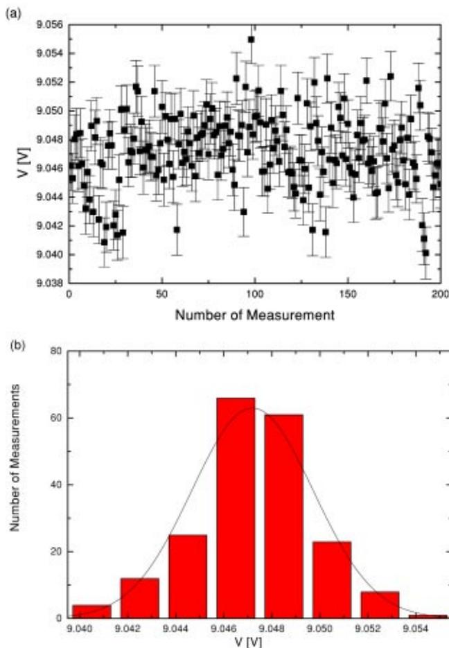
Fig. 3. (a) 200 measurements of the 9 V battery voltage after adding noise and averaging over 10 000 points, in the order that they were obtained. (In all cases  $S_i=0.18$  V and  $S_{N_i}=0.0018$  V.) (b) Histogram of 200 of the 9 V battery voltage dithered data. The mean value is 9.047 V and the standard deviation is 0.002 V.
