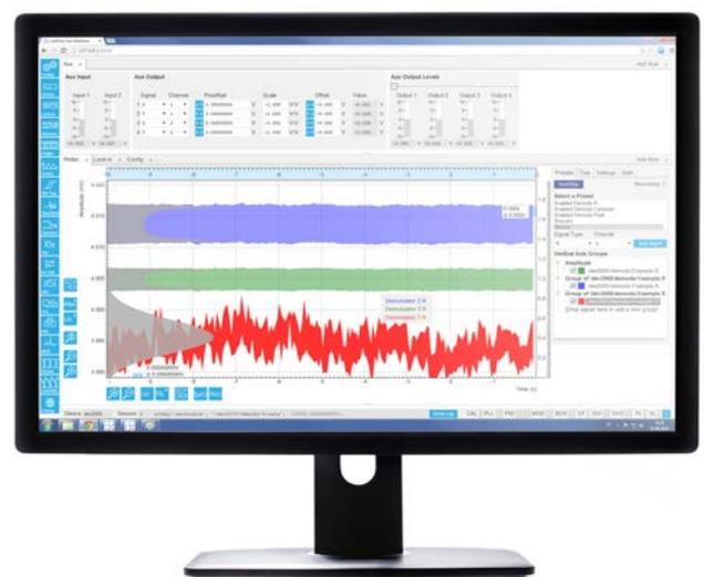
**Figure 15.** The LabOne® user interface of the UHF Lock-in amplifier uses the latest web browser technology. The instrument can be controlled from multiple browser sessions on multiple PCs, tablets, etc. at the same time. Every signal analysis and control tool has a dedicated tab. Some of the functionality is intuitively displayed in form of block diagrams.
