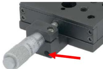
**Do not remove the locking plate and attempt to mount an actuator on that side of the stage.**
