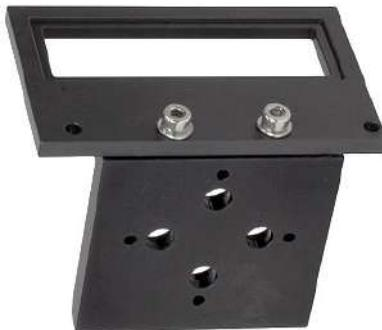
Screw the adapter assembly to the stage using two 1/4"-20, 0.315" long (M6 x 8 mm) cap screws with washers and 4 dowel pins (you may need to use the screws to pull the stages together once you have aligned the dowel pins).
