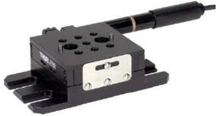
Screw the second MT1(/M)-Z8 with side-mounted motor onto the first one in the orientation shown in the image to the right using two 1/4"-20, 3/8" long (M6 x 10 mm) cap screws.
