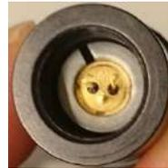
Fix the assembly in the LTN330-A using the black retaining ring (the retaining ring can be tightened using a thin screwdriver). Make sure to use the thick retaining ring and not the one you unscrewed in the previous step. Also, ensure that the laser diode's legs fit through the center hole so they are not damaged, see image to the right.
