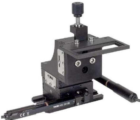
Now, attach the assembled stage on the breadboard at the position depicted in Figure 10 using four 1/4"-20, 3/8" long (M6 x 10 mm) cap screws with washers.
