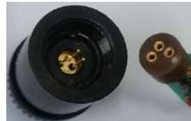
When the diode's legs are in the socket, the cover can be screwed onto the LTN330-A. **Make sure to screw on the part labeled "SR9A-DB9" instead of rotating the part with the printed circuit board!**
