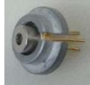
Remove the retaining ring from the LTN330-A housing. Then, insert the diode with the silver retention ring into the LTN330-A.
