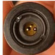
In the next step, insert the laser diode's legs into the socket of the SR9A-DB9. Please be careful in this step to avoid damage to the diode.
