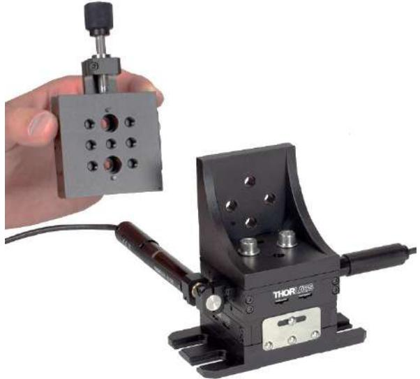
Connect the two pieces of the sample holder using two 8-32", 3/8" long (M4 x 10) mm screws with washers.
