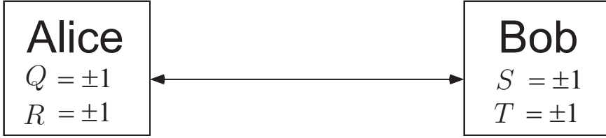
Figure 2.4. Schematic experimental setup for the Bell inequalities. Alice can choose to measure either Q or R , and Bob chooses to measure either S or T . They perform their measurements simultaneously. Alice and Bob are assumed to be far enough apart that performing a measurement on one system can not have any effect on the result of measurements on the other.
